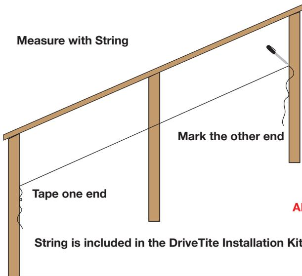
**3** Measure cut length with string and transfer to tape measure.
