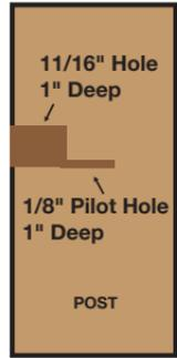
\*When installing in hardwoods, drill 11/16" hole to a depth of 1 1/4" and make the pilot hole 3/16".
