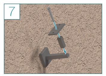
• Using the <sup>1</sup>/<sub>4</sub>" - 20 x 2" screw, attach the top bracket and pillar to the base stem
