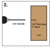
\*When installing in hardwoods, make the pilot hole 3/16".
