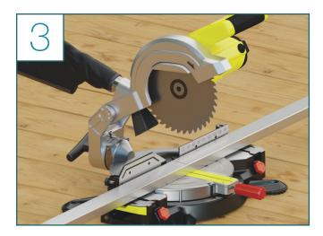
• Using the appropriate blade for the handrail material cut at the mark
