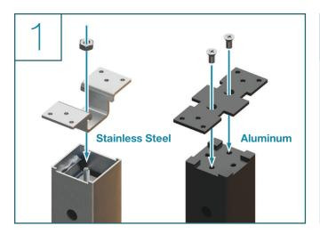
• Attach the handrail brackets to the post tops
